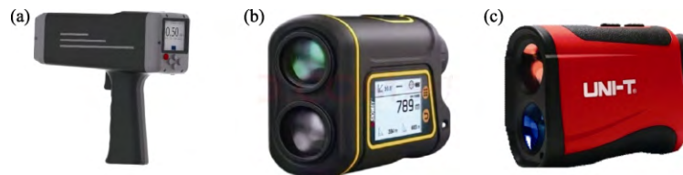
Figure 2 Data acquisition equipment: (a) the handheld radar current meter (RD-60) for measuring stream flow velocity, and two outdoor rangefinders; (b) and (c), used to measure river width and floodplain width
